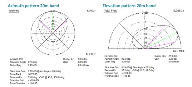
Azimuth pattern at 27 degrees elevation
