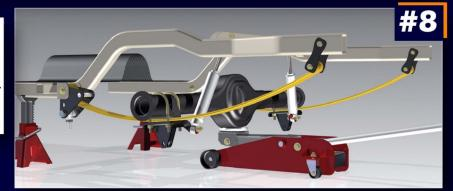
Compress the suspension before attaching transfer links. Apply grease or anti-sieze to rod end threads. Thread both end into link as illustrated. This will ensure that rod ends thread out equally.
