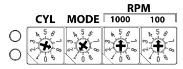
**Note:** Setting a rev limit values less then 1000 RPM requires that the "**1000**" switch be placed in the 0 position. For a maximum rev limit of 10,000 RPM both "**1000**" and "**100**" switches would be in the 0 position.
