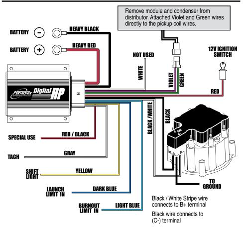
Do not use TACH terminal on HEI. Tach should connect to gray wire.
