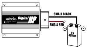
Optional: Programming of the Digital HP can be done before installing. This requires a 9V battery. Attach the small black wire to the battery negative terminal. Program your settings. When finished hold the small red wire on the battery positive terminal. The LEDs will blink indicating the setting is saved.
