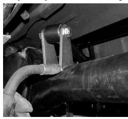
12- Now assemble the shocks per the instructions included, put the bearing ends in and put the springs on. NOTE - anti-seize must be used on the threads of the shock body to prevent galling when you adjust ride height! Install the shocks with the adjustment knobs facing in, and with the springs hand tight. On the lower mount, the spacer goes between the mount and the shock to provide clearance. You MUST use anti-seize on this bolt to prevent galling in the aluminum mount.
