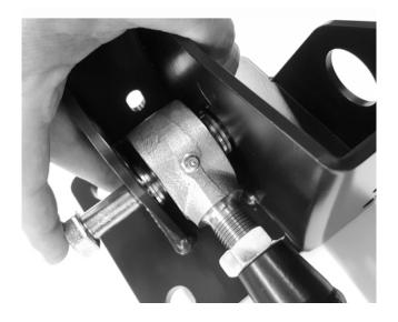
7- Attach the axle plates to the rear axle on the existing mounting pad, using the supplied u-bolts. The plates are positioned so the shock mount faces the front and is inside of the lower link mounting tabs. Then attach the aluminum lower shock mount to the plate. The center two holes are most common. If later you need a higher ride height you can move this bracket to the upper two holes, or if you want the ride height lower you can use the lowest two holes.
