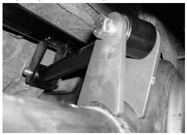
There are longer and shorter tabs included, to offset the angle of the housing. However, various axle housings can differ greatly, and slight grinding may be needed to make the rear bushing line up with the front bushing. This alignment only needs to be close, it does not need to be precisely exact.
