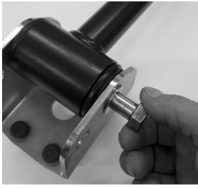
On all flex joint ends, the spacers are installed from the inside as shown below.
