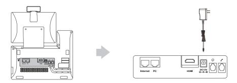
Note: The IP phone should be used with Yealink original power adapter (12V/2A) only. The use of the third-party power adapter may cause the damage to the phone.
