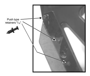
**b)** Repeat steps a) for driver lower door insert (Item A) installation.
