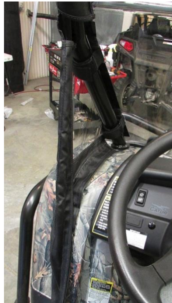
4. Note Velcro on inside edges of side panels along roll cage, & on lower body. Peel off self adhesive backing & stick to roll cage & body.
