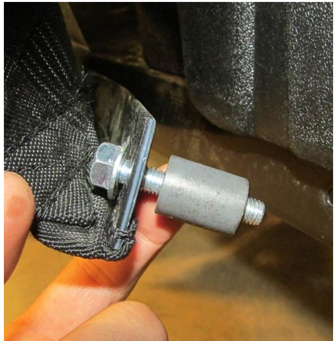
6. The last lower net bolt below the gas tank may have a 1 inch spacer on it. If it does, please remove it and re-fasten the bolt and nut.
