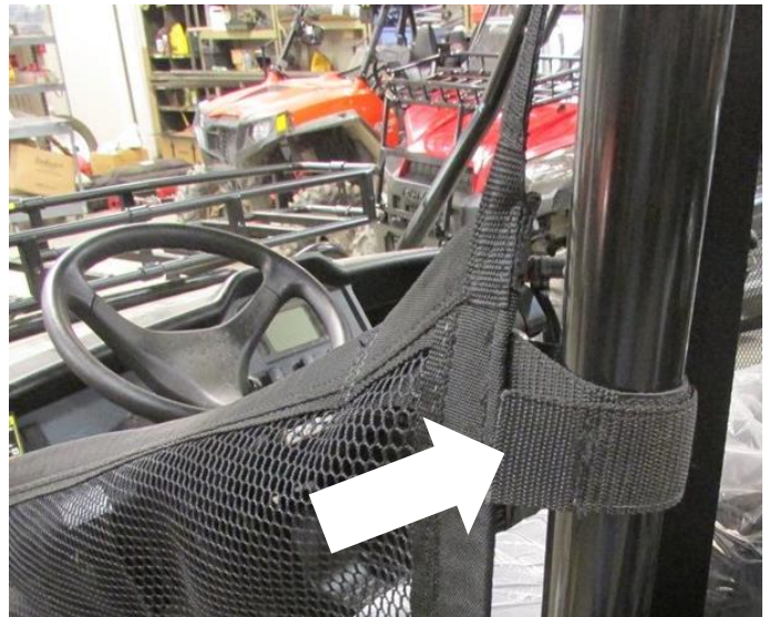
4. Remove this Velcro net strap. After the rear textile is put on you can cut a small slot in the material and re-fasten it. .
