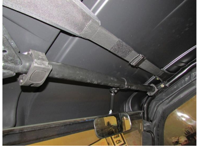
3. Pull straps over roll cage & buckle. Tug on straps to secure the Side Panels tight.
