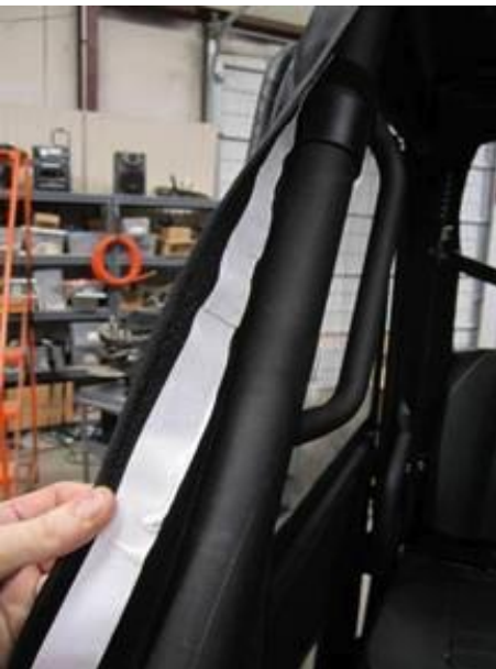
4. Note Velcro on inside edges of side panels along roll cage, & on lower body. Peel off self adhesive backing & stick to roll cage & body.
