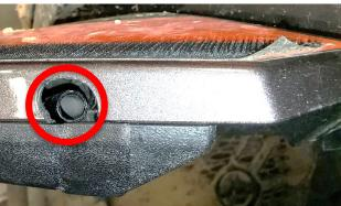
**14.** The Front Mounting Bracket (B) requires the outer panel to be trimmed. Again use a 3/4" drill bit and drill a hole in the outer door panel so that the front door pin may pass through the panel and into the Front Mounting Bracket (B).
