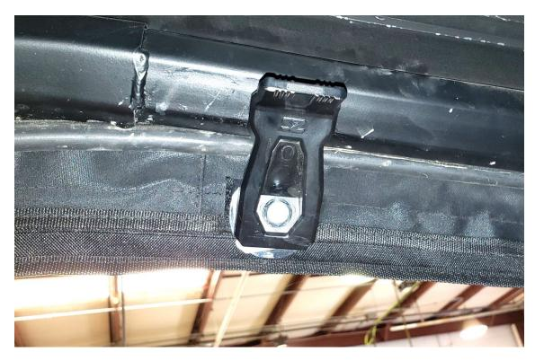
**15.** Your pinned General Upper Door is equipped with an auxiliary close lever (K) located at the top of the door frame. This close lever (K) aids gasket compression and overall door sealing. Simply climb inside the vehicle, close the door, and rotate this lever 180° upward to engage on the ROPS as shown. This will help seal the door and should also be engaged when trailering the vehicle to prevent unwanted door failure due to high wind speeds.
