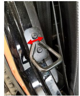
**NOTE** The factory Striker pin can be adjusted if the door is not closing easily because of the added weight and force of the door closing against the gasket
