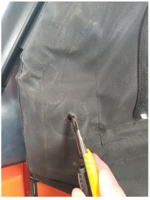
**17.** Using a sharp razor or utility knife, cut the textile so the mirror mounting bolt can pass through.
