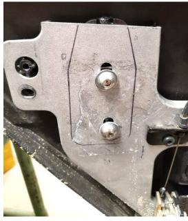
**7.** Insert EZ clip M10 nuts (F) into Rear Mounting bracket (C) as shown. Slide the Rear Mounting Bracket (C) between the aluminum door frame structure and the outer door panel. Use 2 m10x25mm button head bolts and washers thread into the EZ clip nuts (F). The slots in the frame and where the EZ nuts ride will allow for proper alignment of the door pins. Install only finger tight at this time.
