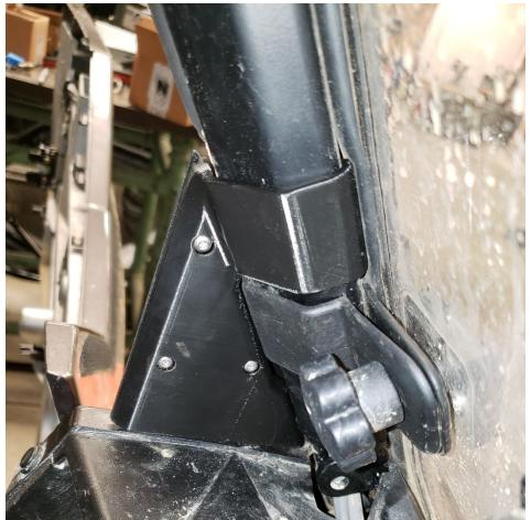
11. Install the front filler panel inner (H) to the front filler panel outer (F) using supplied torx head screws (3 per side) as shown in the pictures above. Install until snug. CAUTION OVER TIGHTENING THESE SCREWS WILL CAUSE DAMAGE TO THE FRONT FILLER PANEL OUTER (F) SCREW BOSSES.
