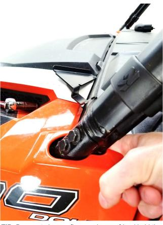
**TIP:** Be sure to keep a finger or have a friend hold the nuts in place or they will fall and possibly be hard to locate. A magnet can be your friend here.
