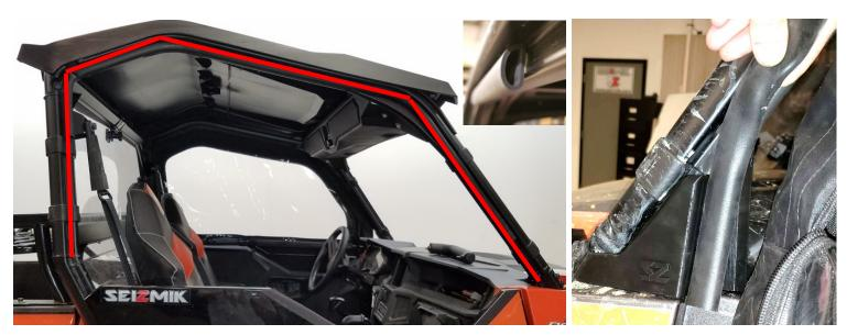
**20.** Clean the highlighted area of the roll cage and filler panel with rubbing alcohol or window cleaner. Adhere the provided gasket into the outer channel of the roll cage as shown by the highlighted area above. Be sure the gasket is oriented the same as the image above.
