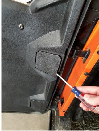
**2.** Use a flat blade screwdriver to remove the hinge adjustment covers to reveal the last two Torx fasteners (top and bottom). Remove the inner door Panel
