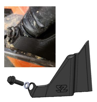
**9.** Install the front filler panel with the front filler panel shims inside the hole as shown above. These act as a crush sleeve for the plastic panel
