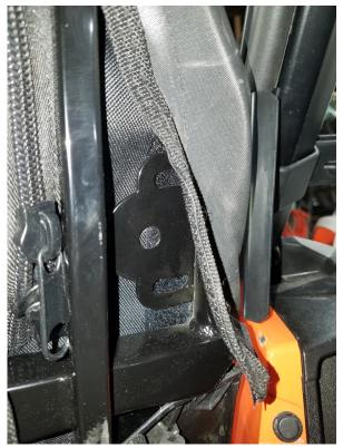
**16.** Locate the mirror mounting bracket on the inside of the door frame. Mark the location of the hole with a punch so that it can be seen on the outside of the door textile.
