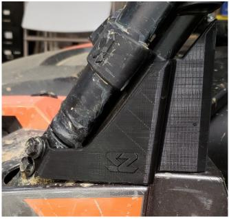
**10.** Re-Torque the Factory Cage bolts to Polaris Spec's.
