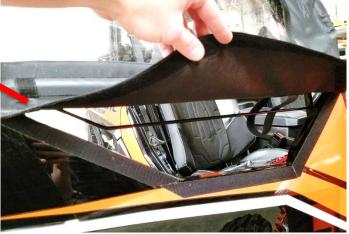
**22.** Cut the Velcro to the correct lengths and adhere to the area marked before and stick the flap down.
