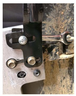
**6.** Re-install the bolt removed in step 4. Then install an M8-25 and locknut with washer in the top hole of the bracket. Install only finger tight at this time.
