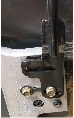
**5.** Insert the front spacer block between the Front Mounting Bracket (B) and the aluminum Polaris door frame.
