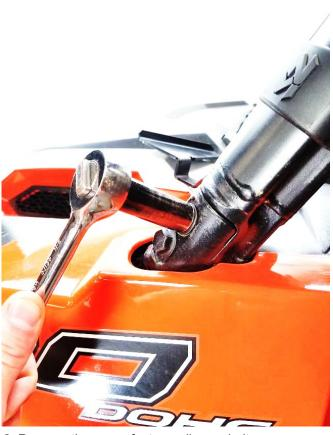
8. Remove the upper factory roll cage bolt.
