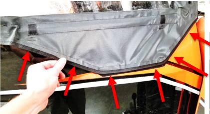
**21.** Lay the Textile Flap over the outer door plastics and mark the location of the outside perimeter. Clean the designated area with rubbing alcohol or window cleaner.
