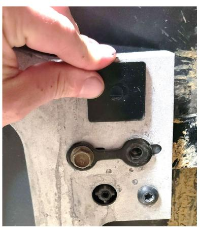
**4.** The front spacer (D) ensures the Front mounting bracket (B) is installed with the correct offset so that the pins on the upper door frame line up with the bracket.
