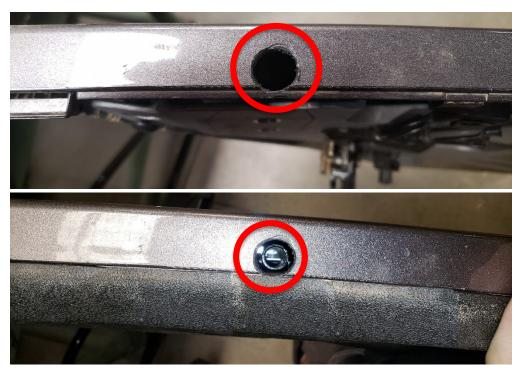
**13.** Use a 3/4" drill bit (or step bit) and drill a hole in the rear of the outer door panel so that the door pins may pass through the panel an into the Rear mounting bracket (D).
