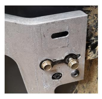
**3.** Remove the upper door hinge mounting bolt closest to the vehicle as shown above (you will re-use this bolt later).
