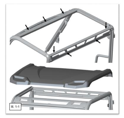
Loosely install two M6 x 25mm Torx Screws (Item #2) on the rear wall of the Roof. The Torx Screws will self tap threads into the OEM holes in the roll cage. Then loosely install two M6 x 25mm Torx Screws (Item #2) and Lock Nuts (Item #4) on the top side of the rear Roof section. Be sure not to cross thread fasteners. (See Illustration 1-2).
