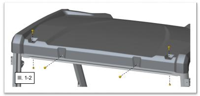
Loosely install three M6 x 25mm Torx Screws (Item #2) and Lock Nuts (Item #4) in the mounting holes towards the center of the Roof. Be sure not to cross thread fasteners. (See Illustration 1-3).
