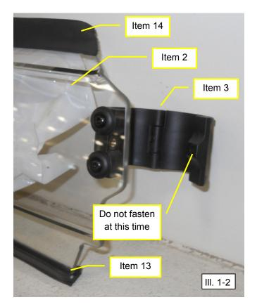
5. Take the Lower Windshield Assembly and position onto the ROPS and against the hood surface. Install and tighten to specification (2) M6 x 18mm Button Head (Item 4) and (2) M6 Lock Washer (Item 5) into the clamp assemblies to secure the clamps around the ROPS. Then tighten to specification the (4) M6 x 18mm Button Heads that secure the clamps to the lower windshield. See Illustration 1-3 and 1-4.
