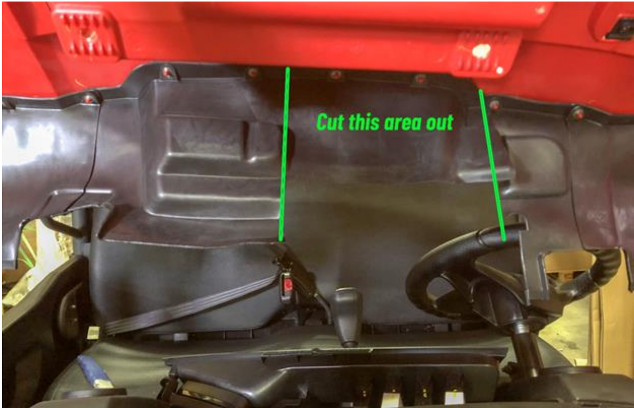
PIC04 – hood panel shimmed up ROPS bars in this picture
