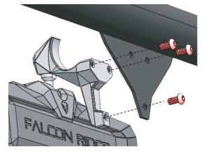
Screw and tighten the M6x16mm button head bolts through the holes to secure the clamp and mirror to the mirror mounting plate.
