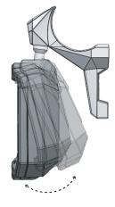
Adjust angle of mirror housing as necessary.
