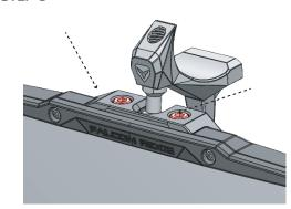
Use these bolts to adjust tension on the ball joint. Clockwise turn will increase tension, Counter-clockwise will decrease tension.
