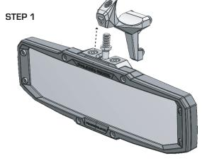
Attach the mirror housing to the Can Am X3 clamp
