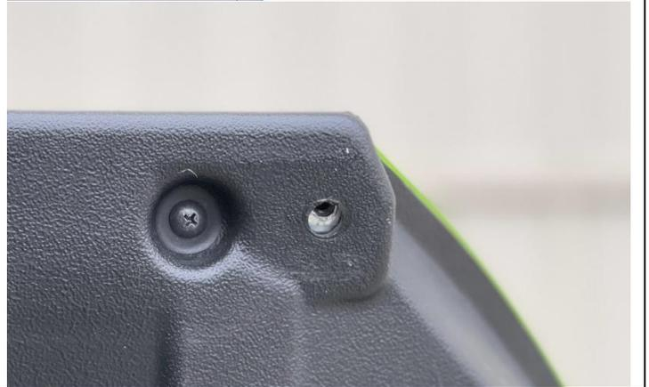
15) Fasten the webbing with metal grommet to the threaded hole at the rear section of the lower door using a M6x20mm Screw and M6 Fender Washer.
