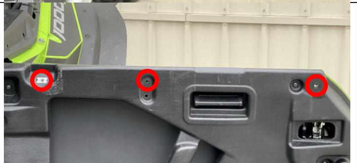
11) Uninstall the two push pin rivets.
