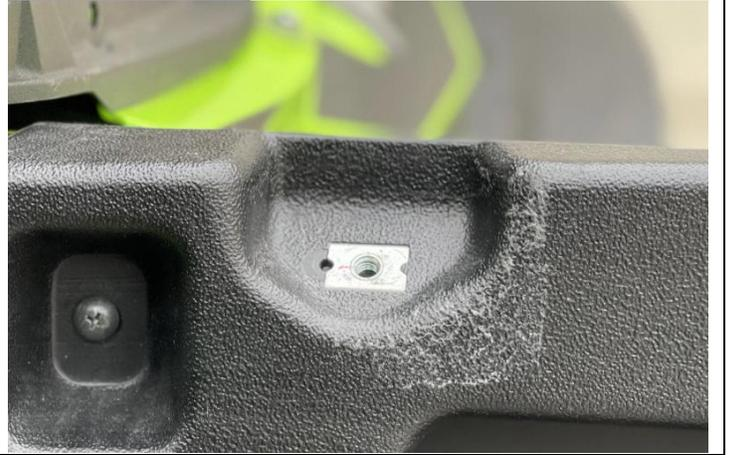
16) The mid bracket overlays a slot shaped indent on the lower plastic door. Adjust to align the lower hole of the bracket close to the center of the indent. Mark the position with an awl and drill a ¼" through hole in the plastic door.
