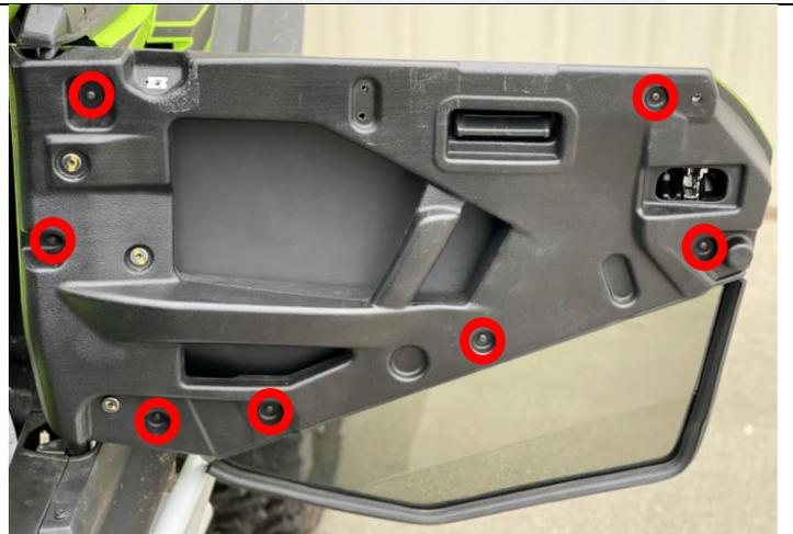
10) Uninstall the 3 fasteners at top edge on the inside of the lower door.
