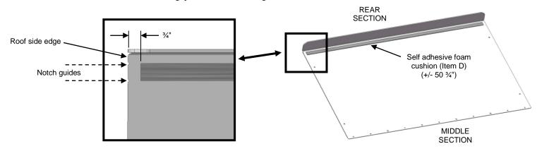
c) Apply the self-adhesive foam cushion (Item E) to the front side of the rear roof (Item B) as shown. For proper installation, the roof must be free of any dust or any other contamination. Using a pen, screwdriver or any other similar pointy tool, pierce through the foam cushion using the rear roof mounting holes as guides (11 locations).
