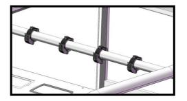
To apply more or less tension to the roll cage, simply rotate the clamp handle from the tension screw as shown below. Over tightening clamps to roll-cage could cause parts failures.
