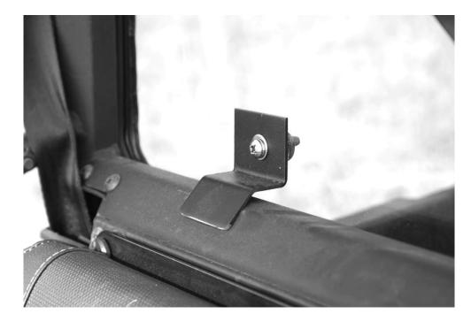
4. Next place the Rear window on the frame of the Prowler and hook the brackets on the bottom of the frame as shown in the photo below. You will need to get someone else to hold the Rear Window in place in order install the remaining brackets.
