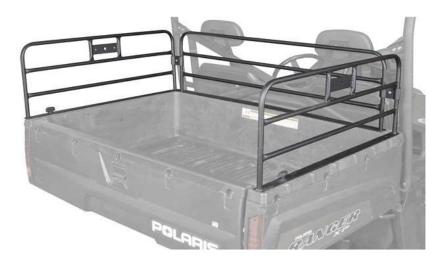
The Ranger BR 500 Bed Rail Installation Kit fits Ranger Mid-Size Models 400, 500, 570, EV & 800. The BR-800 Kit fits Ranger Full-Size Models XP700, 800 & 900. The Kit comes with 2x Side Rails, a Front Rail, 4x Corner Brackets, 2x 5/16-18 Bolt Sets (Bolt, Lock Washer, 2x Flat Washer, and T- Knob) and 5x Anchor Assemblies.
