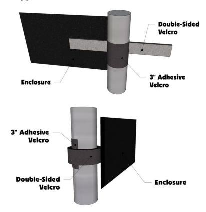
7. Begin installation of the Door Panels by hanging them from the Double-Sided Strips along the top of the doors. Hold the door up and mark where each strip is and wrap a 3" adhesive strip around the roll cage. Now hang the door up and it will be in place to install the rest of the Velcro for the door. See photo below:
