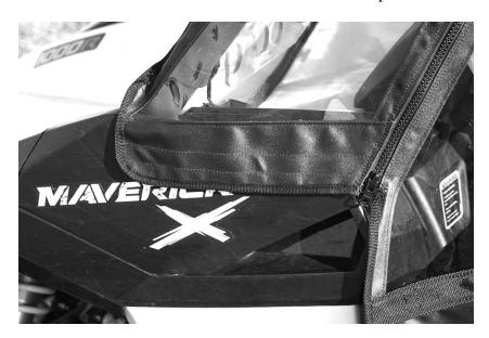
10. The rear of the door has two double-sided Velcro tabs that will attach to the first bar towards the rear of the vehicle. Apply the 6" and 12" adhesive Velcro strips between the horizontal bars facing the rear of the vehicle. (NOTE: You may need to cut the adhesive strips down to fit.) Then attach the double-sided tabs to the adhesive strips as shown in the photo below.
