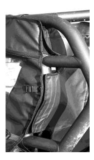
11. Next work your way around the bottom of the door panel and install a snap stud for every snap on the Door Panel. TIP: You may find it easier to snap the screw stud into the socket on the door first and then pull the Door Panel to the position it should be in and push the screw into the plastic to mark its position. Then remove the screw stud from the socket and drive it into the plastic. See Photo Below:
