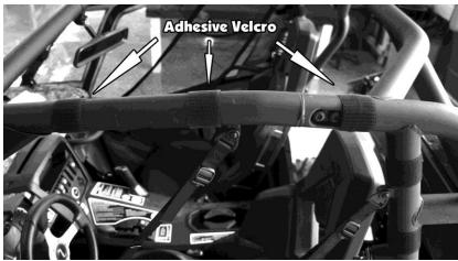
8. Now move around the door and attach the remaining Velcro strips in the same manner. Down the front of the door place the edge of the door against the side of the windshield and run the Velcro strips under it with the 3" adhesive Velcro on the inside of the roll cage.
