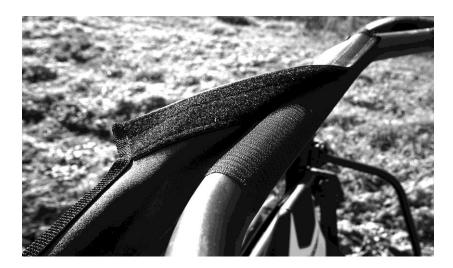
4. Next take the 20" adhesive Velcro strips and run it down the back of the roll cage facing towards the rear of the vehicle. Start at the bottom and work your way up the bar. See photo below.
