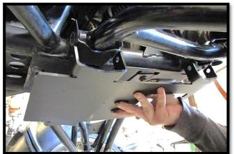
5. Replace the factory hardware with **10mmx110mm hex bolts**, **10mm flat washers**, and **10mm lock nuts**. Fasten hardware to factory specifications.
