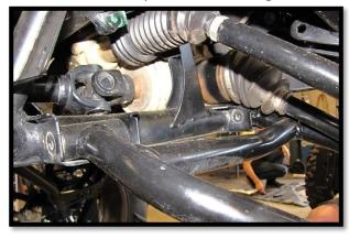
4. Place the frame stiffener plate **117P** to the frame and align the frame tab holes.
