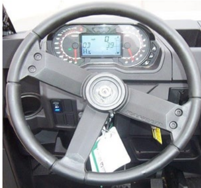
A) When the steering is zeroed, check the steering wheel to make sure that it is properly positioned.
