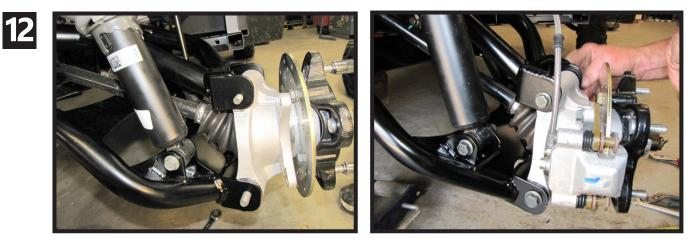
Attach the lower arm to the hub assembly using factory hardware. DO NOT FORGET WASHERS.
