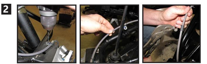
Drill out the factory p-clamps until they snap off, then remove the clamps.
