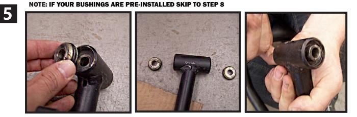
Use caution when removing the bushing from the collar, there is a stop built into the factory arm that prevents the bushing from pushing out when installed. Because of this, the bushing must be pushed out from the opposite side!! A flat punch or press is recommended to remove the bushings.
