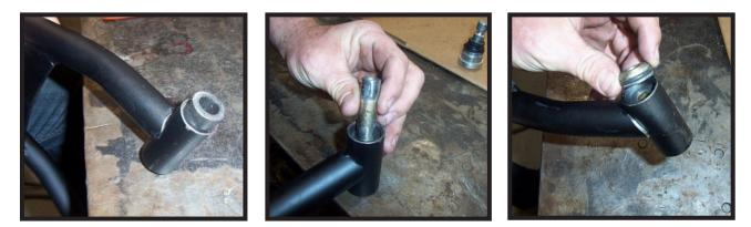
NOTE: Applying grease to the bushings and sleeves will make the installation easier. NOTE: Once the bushing is inserted, you will need to use a socket to help press it in all the way.
