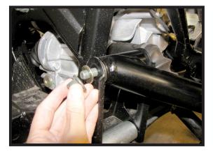
Once bushings are installed, **connect the new upper arm** to the frame using the factory hardware. **DO NOT FORGET WASHERS.**
