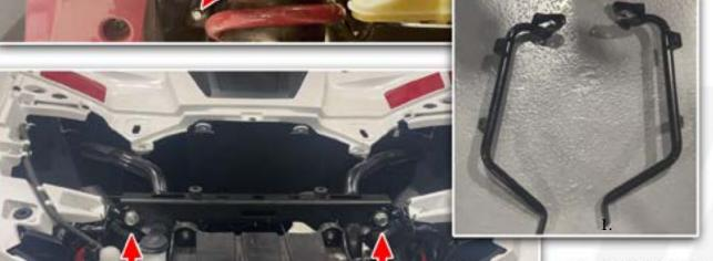
NEXT, REMOVE THE TWO FACTORY SHOCK BOLTS. AND MOVE THE SHOCKS ASIDE.
