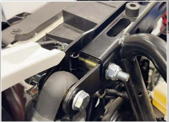
ENSURE THAT EVERYTHING FITS PROPERLY THEN TIGHTEN TO SPEC REINSTALL THE TWO BRACKETS YOU PREVIOUSLY REMOVED, REINSTALL WHEELS AND LOWER THE JACK.
