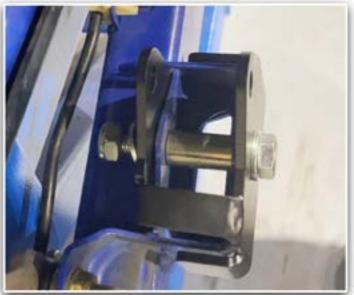
NEXT, INSTALL THE SHOCK. ONCE THE SHOCK IS LINED UP INSERT A 12MX70MM BOLT WITH A WASHER THROUGH THE SHOCK AND THE AA SPACER. ONCE THROUGH PUT ANOTHER WASHER ON THE END THEN A 12M NUT.
