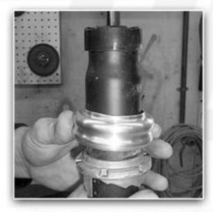
ONCE YOU HAVE REMOVED THE SPRING, PLACE THE LIFT BRACKET ONTO THE SHOCK **BODY WITH THE SPRING ALIGNMENT RIDE** FACING TOWARD THE PISTON.
