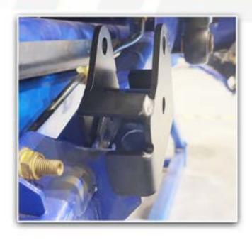
SET THE LOWER LIFT BRACKET OVER THE SHOCK TAB ON THE TRAILING ARM LIKE IN THE PICTURE TO THE LEFT.
