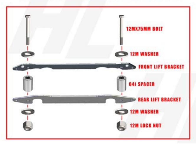
NOW USING THE PROVIDED M12X70MM BOLTS AND NUTS WITH WASHERS ON EACH END INSTALL THE SHOCKS.
