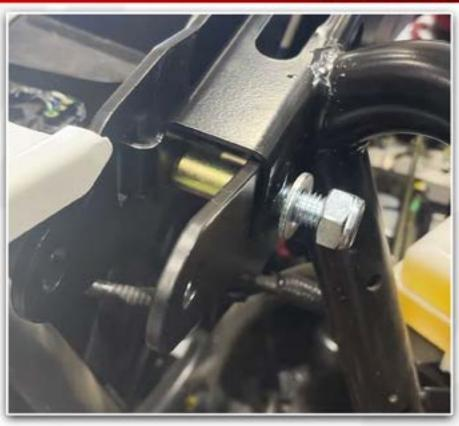
\*THE SPACER IS SET BETWEEN THE TWO BRACKETS INSIDE THE FRAME CHANNEL.
