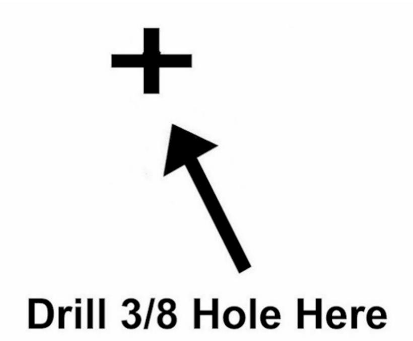
Cut out template. Tape to underside of dash panel below cup holder. Mark hole centers on panel. Remove template. Drill 3/8" holes. Please Note: Before you drill please check the other side of firewall/dash for anything that may interfere with the placement of the holes. We will not be held responsible for holes being drilled in the incorrect place. www.utvpartsandaccessories.com 1 800 596 0785
