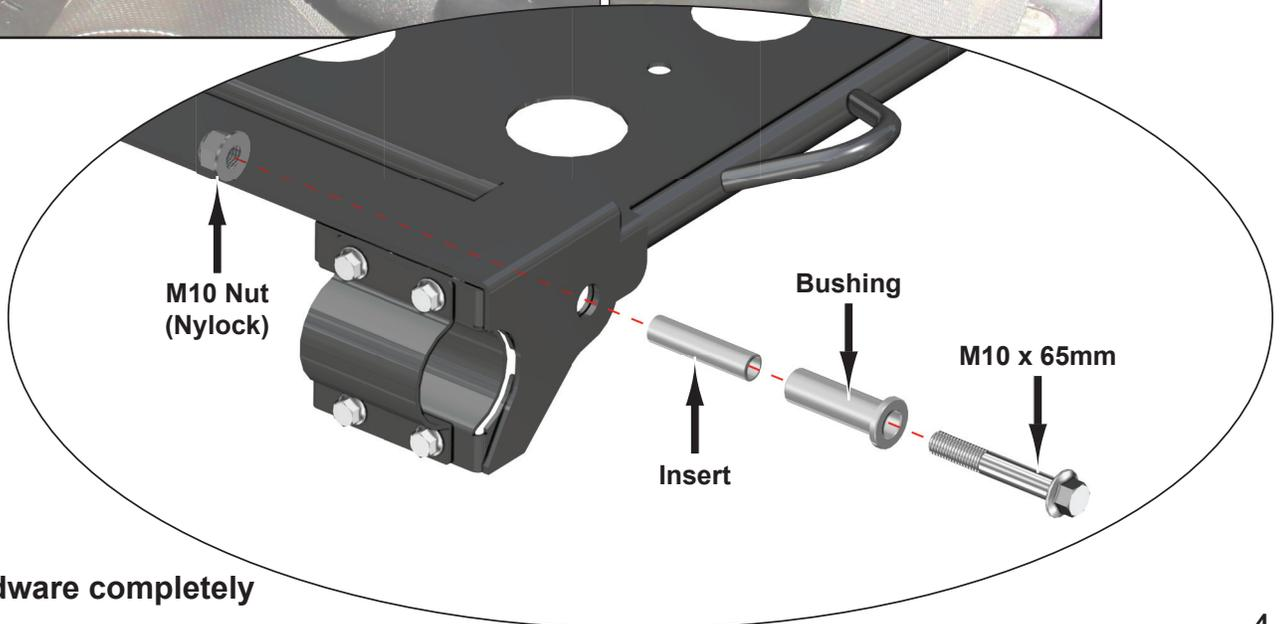
**tighten hardware completely**
