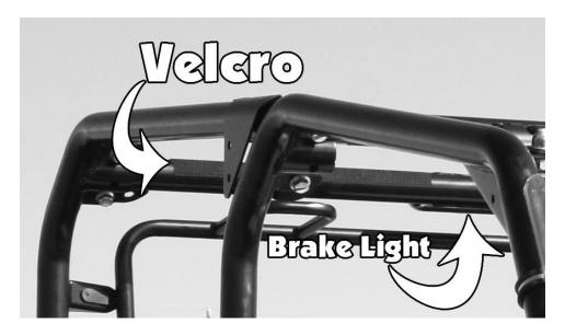
6. After placing the Velcro on the roll cage, attach the rear window. Across the top of the rear window is a cutout for the brake light, line this cutout up with the brake light and attach the rear window to the adhesive Velcro. See Photos Below:
