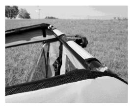
5. Next step is to attach the sides of the rear window to the roll cage. There are 5 strips of double-sided Velcro sewn perpendicular to the edge of the panel. Take the 6" adhesive Velcro strips and wrap them around the bars where each double-Sided Velcro strip lines up. Then wrap the double-sided Velcro around the adhesive strip on the bar. The photos below show how this works.
