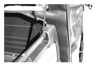
4. Now pull the strap up and run them through the buckles sewn into the rear corners of the Top Cap as shown in the photos below.
