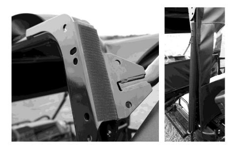
7. Now it's time to work on the bottom of the door. The front part has two strips of Velcro that goes on the front fender. The outer portion of the door has Velcro sewn to the bottom of it and will attach flat to the top of the fender. The bottom front section of the door has a strip of Velcro that attaches to the fender facing the rear of the vehicle. Photos below shows where the Velcro strips should be.
