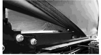
10. Next attach a piece of 26" adhesive Velcro across the top bar, it should be placed on the top slightly angled towards the front of the vehicle. See Photo below.
