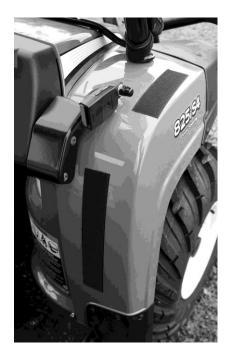
8. Lastly place an adhesive Velcro strip along the side of the floor as shown below.
