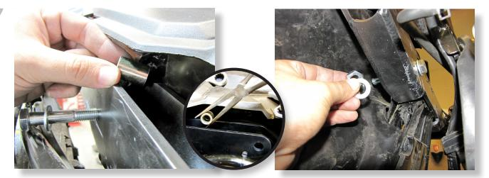
Insert the **bolt** through the **spacer 39C.** Use a pair of pliers if it is difficult fitting it between the bracket.
