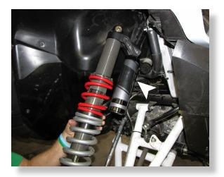
Reinstall the shock back on to the unit.
