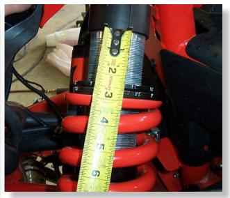
Run the Spanner nut back out to the preset position that was marked before the install.
