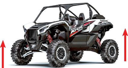
Place a **jack** under the **FRONT** center of the SXS and lift until the weight is off the suspension. Ensure that the vehicle is properly secured, so that it is stable on the jack.
