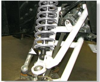
Secure the lower portion of the shock to the control arm using factory hardware.
