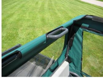
• Now hang the cab from these spots by attaching the Velcro tabs sewn to the cab enclosure in these spots. It may be necessary to remove and reattach the tabs until the cab is centered correctly.
