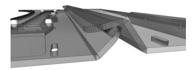
9. The diagram below shows the proper placement sequence of the hardware. Use the 1" bolts for this application. Install each one loosely at first; after you have centered the windshield and are satisfied with exact placement, then you may snug the thumbnuts appropriately.
