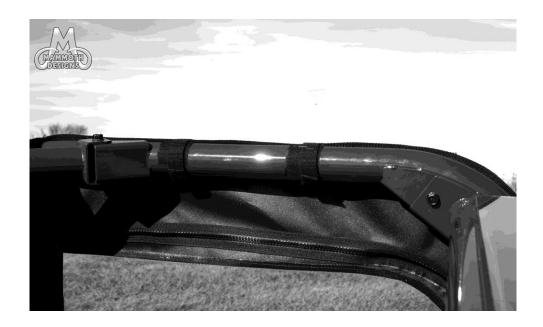
9. The back of the door has a cutout with a bungee cord across it. This spot has to go around the metal block sticking out the sides of the vehicle. Placing the door here helps line up the rest of the door so all the Velcro goes where they need to. See photo below:
