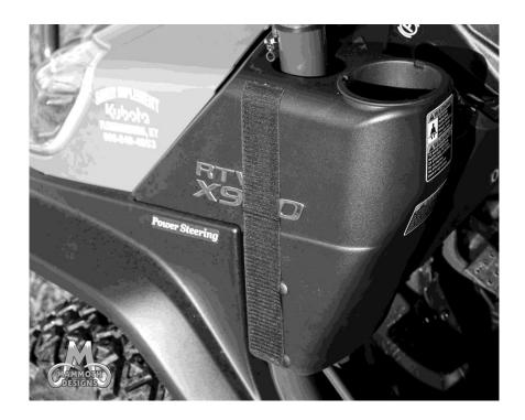
13. Last step is to attach the rear of the door panel to the rear window and to the roll cage just under the rear window. The two top tabs will attach right to the Velcro down the sides of the rear window. The bottom tab will attach directly to the roll cage using an 8" adhesive Velcro strip. See photo Below:
