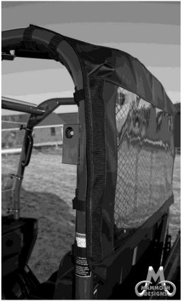
8. Now move on to the door panels. The top and front of the door has the same double-sided strips as the rear window and attaches the same way. See photo below:
