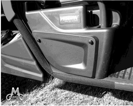
12. Next take the 14" adhesive Velcro strips and attach them to the vehicle just under where the roll cage ends down the front. See photo below:
