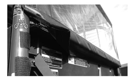
5. Now pull the rear window up and attach it to the top bar across the back of the roll cage. The top and sides of the rear window has double-sided Velcro sewn along the edges. At each of these strips you will place a 3" adhesive Velcro strip on the inside of the bar to hold the double-sided Velcro in place. The diagram below shows how to place the Velcro.
