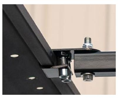
4. Place header panel clamp over the rearward edge of the panel as shown and fasten the slider tube to the clamp using the supplied M10x55 bolt and nut. Snug the x2 M10 socket head bolts on the header panel clamp but keep enough slack so that the assembly can be moved left or right as seen in the next step.
