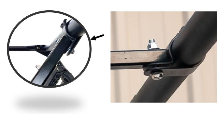
3. Take the gun grip assembly with slider tube inserted (tighten rattle prevention bolt so the slider tube doesn't fall out) and mount to the p clamp using the supplied M10x55 bolt and nut. Keep loose at this time.
