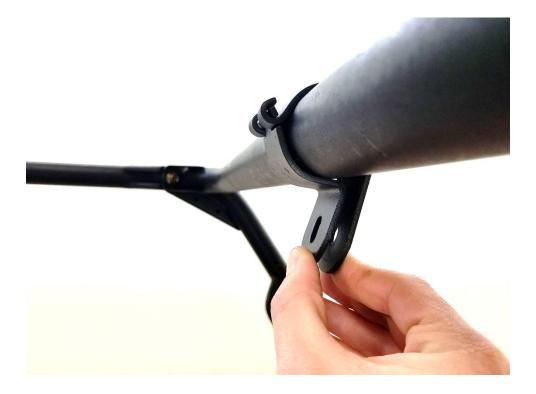
2. Place a metal P clamp around the rear upper roll cage tube.
