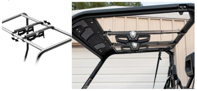
5. Mount the second gun grip assembly just like the first. Adjust the width between the two gun grip assemblies to best fit your guns. After the desired width is found, tighten the M10x55 bolt and nut, as well as the M10 socket head bolts on the header panel clamps to lock the gun grips assemblies in the desired location.
