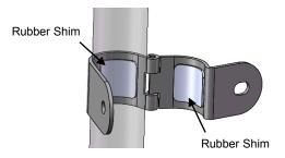
Use a shim on each half to adapt the 1.75" roll cage clamp down to 1.5" and do the same to adapt the 2" clamp down to 1.79" (Honda Pioneer)
