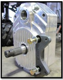
d. Slide a 1/2" flat washer onto (4) 1/2 x 4-1/2" bolts and insert them into the remaining four holes of the box.
