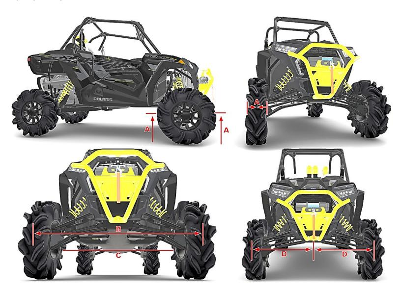
Place the machine on a smooth level surface and set the steering wheel in a 'straight ahead' position. Secure the steering wheel in this position.
