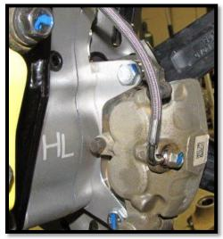
h. Next, pull any extra slack out from the caliper to under the seat. Then re-use your **factory p-clamps** to secure the new brake lines to the trailing arms. Insert a **6mm x 12mm screw** through each clamp and fasten them. **Do not over-torque!**
