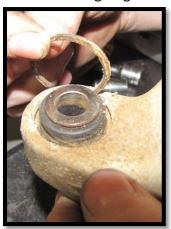
c. On the other side of the joint, the knuckle has a built in stop. Find a socket or tool to fit the inner diameter of the stop. Then use a press or a vise to remove the joints.
