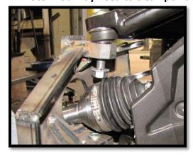
Position the lower ball joint into the lower ball joint mounting bracket on the backing plate.
