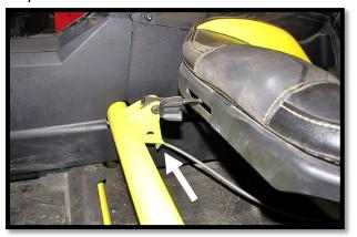
j. Slide a **p-clamp (WL-CLAMP-12)** over the brake line. Secure it to the rear backing plate using a **5mm x 20mm bolt** through the clamp and backing plate, followed by a **5mm washer** and **5mm lock nut.**
