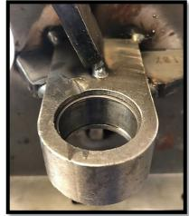
h. Find a 13/16 socket or pipe to press the joints in. We recommend applying a small amount of grease to the joint, then place it <u>straight</u> into the bracket. Use a press or vise to press it in until it stops at the retaining ring.
