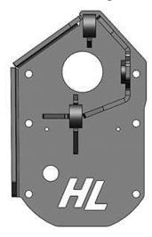
g. The backing plate brackets do not have a built in stop like the factory knuckle. So first you will need to place and snap in a **retaining ring 115M** into one the grooves of each bracket. These will create a stop when you press the joints in.
