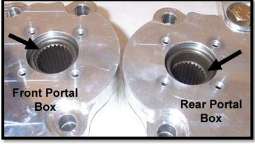
c. Find caliper mounting bracket **PGLC-BCB-106N** and place it in the corresponding fitted <u>FRONT</u> section of the portal box. Then insert a **1/2** x **4-3/4" bolt** and **1/2" washer** into the bracket holes & box.
