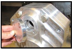
c. Find caliper mounting bracket **PGLC-BCB-1180** and place it in the corresponding fitted <u>REAR</u> section of the portal box. Then insert a **1/2** x **4-3/4" bolt** and **1/2" washer** into the bracket holes & box.
