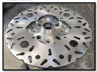
g. Slide a 3/8" lock washer onto (4) 3/8 x 1-1/4" hex head bolts. Apply LOCTITE (RED) to each screw. Insert them through the rotor, the spacers, and then into the hub. Tighten and torque. (9/16) [45 ft lbs]
