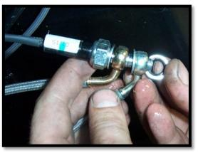
c. Install the new longer brake line 107A to the banjo bolt. Run the line back through the frame and to the (PA) side hub.
