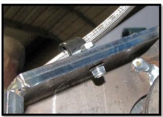
i. Use the factory A-arm clips and the supplied **zip ties** to reposition the brake lines, then fasten the brake line back to the caliper. **Make sure there's no binding in the lines, even at full turn.**
