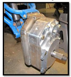
d. Loosely fasten the all four bolts with 1/2" flat washers and 1/2" lock nuts. Recheck all parts that were used and make sure everything fits correctly, and then go ahead and tighten and torque all bolts. (3/4)[105 ft lbs]
