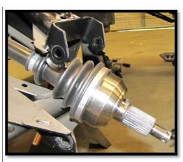
f. While you have the knuckle removed and have more access to the lower arm. You will need to drill/remove the rivet of the p-clamp on the lower factory arm (Or you can simply cut the clamp if you don't want to re-use it). Doing this now will make the new rear brake line installation easier later in the instructions.
