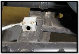
c. Install the new **70"** rear right (pass. side) brake line to the t-block. It will need to be routed down the same passage where the factory line was.
