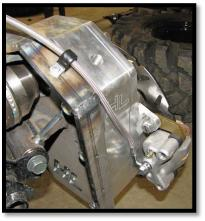
g. Secure the brake lines by using the provided **zip ties**. Make sure there is no binding in the lines once they are secured. (Re-using the factory clamps is optional, but you may need new hardware)
