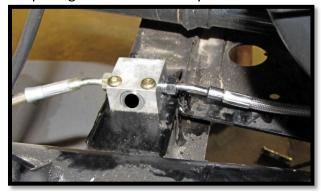
d. Before installing the new **60" rear left** (driver side). First install the 3/8 adapter. The arched end should face out once installed. Now attach the brake line to the adapter.
