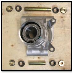
c. Insert the bushings, pivot tubes, and pivot caps into the collars of the **rear right backing plate** (**101J-R**). **NOTE**: We recommend applying good water-resistant grease to the bushings and especially the pivot tube. This will help prevent excessive friction & wear plus add longevity to the life of the bushings and pivot tube.
