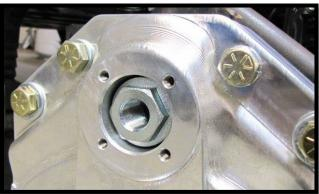
c. Align the portal box lid cap & gasket. Use the 1/4-20 x 3/4" screws and install to the box. (3/16)[8 ft lbs]
