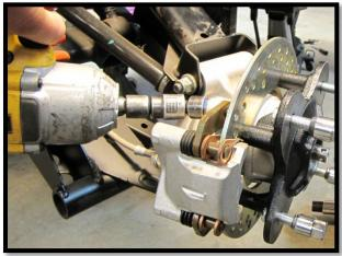
b. Remove the caliper from the rear hub. It is not necessary to remove the brake line from the caliper at this time. Leave the brake hose attached to the caliper and hang the calipers out of the way. Take precautions to ensure the brake hose isn't stretched or pinched.
