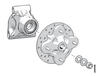
Remove the cotter pin and castle nut (27mm) on the rear axles, then remove the brake rotor assembly.
