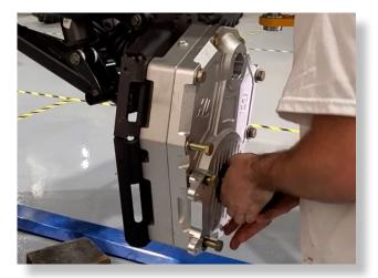
Apply water-resistant grease to the drive splines. Be sure to apply product all around the outer edge as well.
