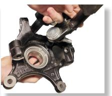
Remove axle, then disconnect the **Lower ball joint** by removing the **nut** at the knuckle. **(18mm)**
