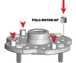
Install the rotor and secure it to the hub by applying LOCTITE (RED) to the (4) 3/8 x 1-1/4" hex head bolts & (4) 3/8 lock washer. (7/32) [45 ft lbs]
