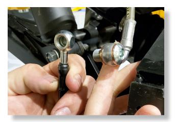
Locate the propper BRAKE LINE EXTENSION. Using the supplied button head hex drive banjo bolt, connect the STOCK BRAKE LINE to the BLIND-END BRAKE LINE EXTENSION. Ensure the copper washers are on each side of the banjo fitting.
