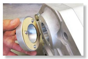
Remove the  $1/4-20 \ge 3/4$ " screws & cap/gasket from the lid of the FRONT portal box.
