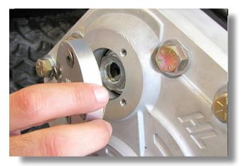
Align the portal box lid cap & gasket. Use the 1/4-20 x 3/4" screws to secure the cap to the portal box. [8 ft lbs]
