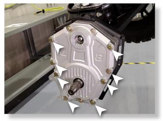
Loosely fasten all (8) bolts with 1/2" flat washers and 1/2" lock nuts. Ensure parts fit correctly then torque. (3/4) [105 ft lbs]
