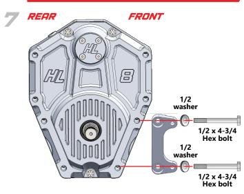
Install the **115N caliper bracket** facing the **FRONT** of the vehicle.
