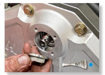
With the portal box installed, apply LOCTITE (BLUE) to the supplied M18 axle nut PGLC-AXNUT-2 and torque onto the drive shaft axle. (30mm) [20 ft lbs]
