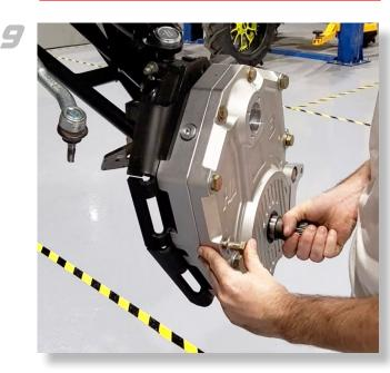
Apply water-resistant grease to the drive splines. Be sure to apply product all around the outer edge as well.
