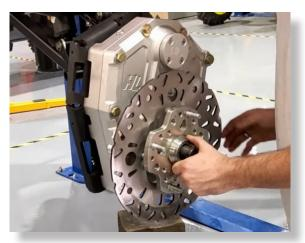
Apply waterproof grease to the spindle splines and slide the brake rotor onto the spindle shaft. Slide on the 30mm lock washer, 30mm castle nut. (46mm) [Min 120 ft lbs]
