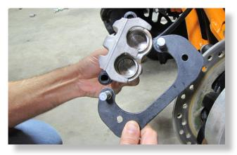
Install the supplied hanger bracket (85X) to the caliper. REINSTALL BRAKE PADS.
