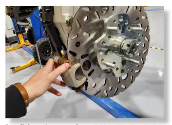
Install the caliper onto the portal box. Use the stock bolts to secure the caliper to the bracket [30 ft lbs].
