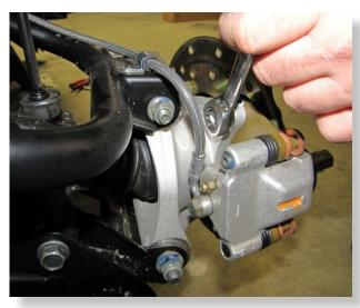
Remove the caliper by removing the (2) stock mounting bolts from the knuckle. (15mm)
