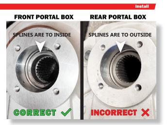
NOTE: On the FRONT portal boxes, the drive gear splines should be recessed to accommodate the shorter front drive shaft splines.
