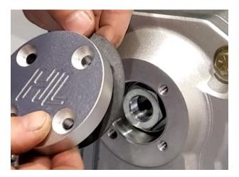
Align the portal box lid cap & gasket. Use the 1/4-20 x 3/4" screws to secure the cap to the portal box. [8 ft lbs]
