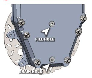
**Use SAE 80W-90 oil.** This gear lubricant is designed for gears operating under severe temperature and load conditions. **SAE 80W-90** viscosity grade offers extended performance.
