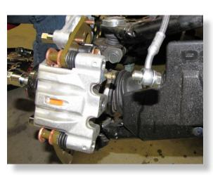
Disconnect the **stock brake line from the caliper**, if you have not done so already. Have a container ready to collect fluid.
