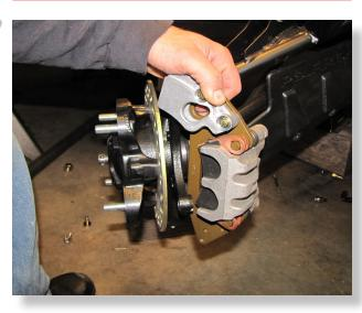
Remove the caliper by removing the (2) stock mounting bolts (15mm) Remove the front mud scraper (8mm). KEEP ALL FACTORY HARDWARE.
