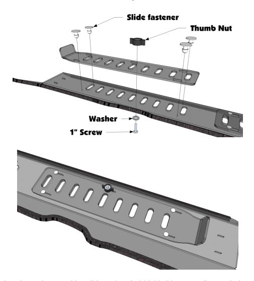
• Next take the bent Lexan brace and install it on the windshield. Please see diagram Below.
