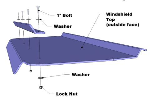
5. Now you are ready to place the windshield on the Ranger and attach to the outside of the roll cage. NOTE: THE BEND AT THE TOP OF THE WINDSHIELD SHOULD GO BELOW THE TOP TUBE.
