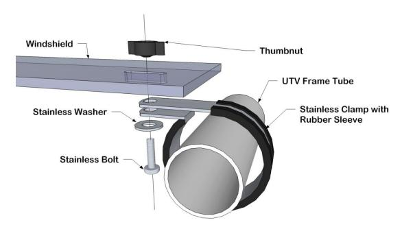
5. Now Place the two halves onto the frame as shown below. (diagram not Ranger)
