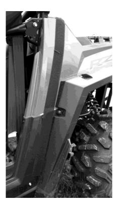
11. Next take the front of the door and tuck it inside the vehicle. There are three snaps that will go on the inner panel. NOTE: it helps to place the screw snaps into the sockets on the cabs first, then starting at the top one, push them into the plastic so a small dimple is left behind. Then pull the screw snap back out and screw it into the plastic where the mark was made. See photo below
