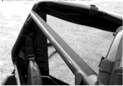
b. The sides of the Rear Window have Velcro sewn down the length of it.. For these you will take the two 20" adhesive Velcro strips and attach them down the rear bars facing the rear of the vehicle. Then attach the sides of the rear window to the bar as shown in the photo on the next page.
