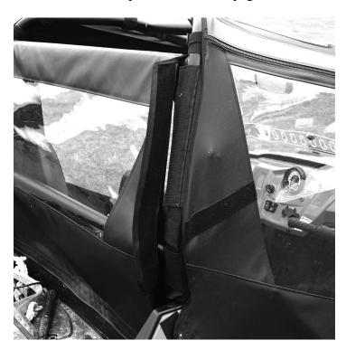
c. Finally take the 42" adhesive Velcro strip and attach the bottom of the rear window to the inside of the rear cargo area. See Photo Below:
