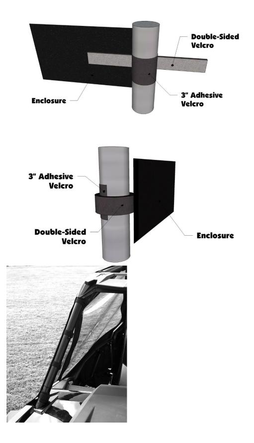
b. After installing the double-sided strips move to the top of the door and attach the 37" adhesive hook strip starting at the front and work it on the bar towards the rear. The strip will start on the side of the bar and end up on top of the bar at the rear. See Photo Below:
