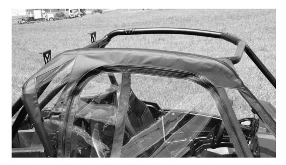
c. Next attach the bottom of the door to the plastic doors on the RZR. Use the 30" adhesive strip and one of the 14" adhesive strip to attach the soft door to the plastic. Then use another 14" adhesive strip to attach the bottom of the front wing to the side of the hood. See photo below:
