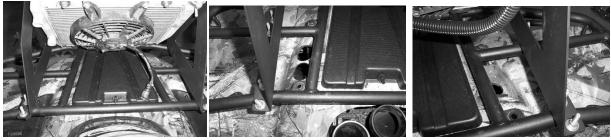
8. Insert the hoses through the holes, cut enough hose to connect the inlet and outlet hoses to the stock hoses you left connected to the ATV engine. Clamp hoses to the radiator using clamps provided.
