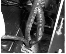
18. Wrap all hoses with the large wire loom and wrap together the overflow bottle lines and wires in the larger wire loom to protect it from cutting and vibration.
