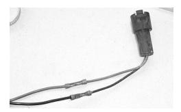
16. Wrap the wires in black tape, and run it through the <sup>1</sup>/<sub>4</sub>" wire loom. Connect the end back to the connector under the plastic,
