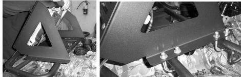
Note: On the left side of the rack you will drill two openings, one for the inlet hose and one for the outlet hose. On the right side you drill a hole using a  $1\frac{1}{2}$  hole saw for the over flow bottle intake and vent lines and the fan wires.
