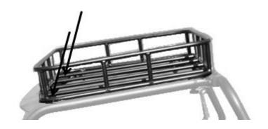
Insert (provided) Bolts, Washers and Lock-Nuts in front corners where the Torx Bolts were removed- do not completely tighten down yet.
