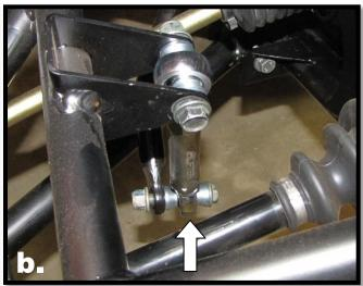
c. Once you have determined the correct position that fits with your setup, adjust & fasten the heims & jam nuts accordingly to the correct length.
