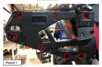
Remove door cover from the door frame by removing eight OEM screws as shown in Picture 1. Retain as they will be reused.
