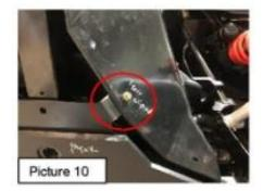
K. Locate one supplied 1/20 x 1" serrated flange bolt. Insert the 1" bolt through the front fender well into the u-nut on the tab. See Picture 10.
