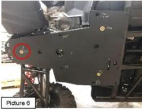
G. Locate one supplied 1/20 x 1" serrated flange bolt, one supplied bowl washer, and one supplied 1/20 t-nut. Insert the 1" bolt and washer into the rear hole of Panel C and secure with the 1/20 t-nut. The t-nut can be accessed from the rear of the vehicle. See Picture 6. Loosely tighten.
