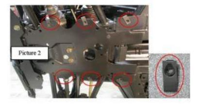
B. Locate six supplied ¼-20 u-nuts from the supplied bolt pack. Insert these into the OEM holes between the front a-arms. See Picture 2.
