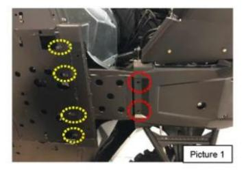
B. Locate four supplied 1/4-20 u-nuts. Insert these as shown in Picture 1 (shown in YELLOW).
