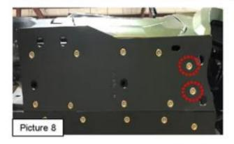
Repeat Steps G and H for Panel E. Securely tighten all fasteners. See Picture 9 for final install.
