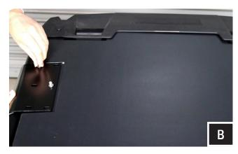
B. While holding the enclosure securely toward the front crossbar of the cage, loosely install the 2 brackets using the screws provided.
