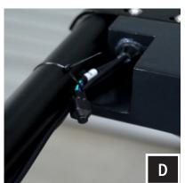
D. Using the zip ties provided, route the Power/Ground loom to the battery location away from any moving parts or sharp metal. NOTE: The 4 pin short cable is for additional speakers (WP-RZ30+2) and the 4 pin long cable is for adding an SSV Works Powered Subwoofer (Part# WP-RZ3GBS10 or WP-RZ3BSS10)
